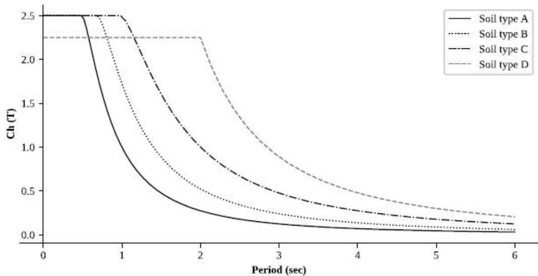
Fig : Spectral Shape Factor,  $Ch(T)$  for Equivalent Static Method
