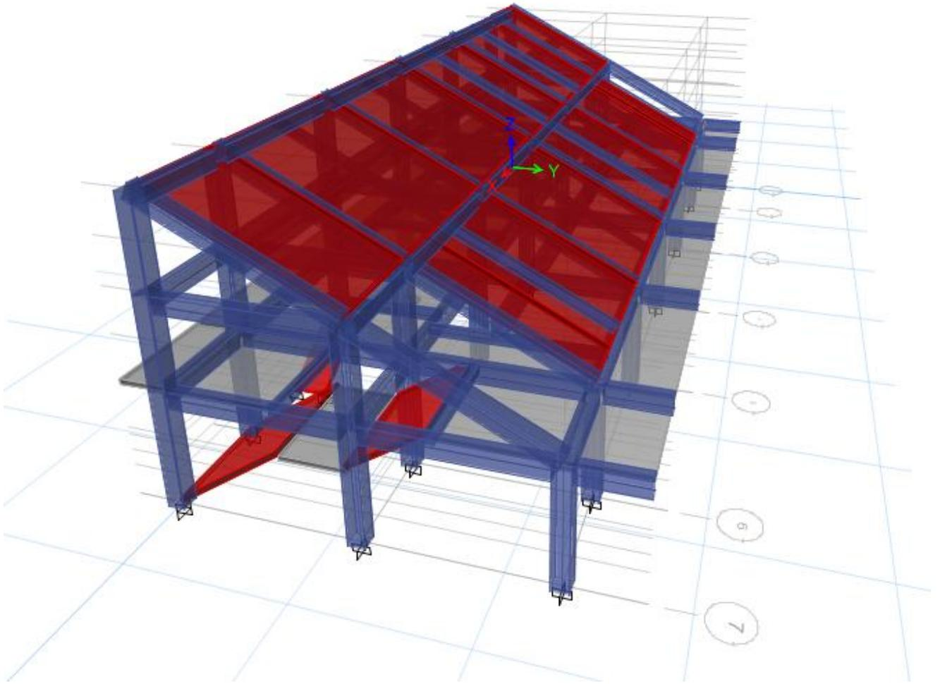
*Figure 2: Finite Elemental Modeling in ETABS V19 (Block A 1 & 3)*
