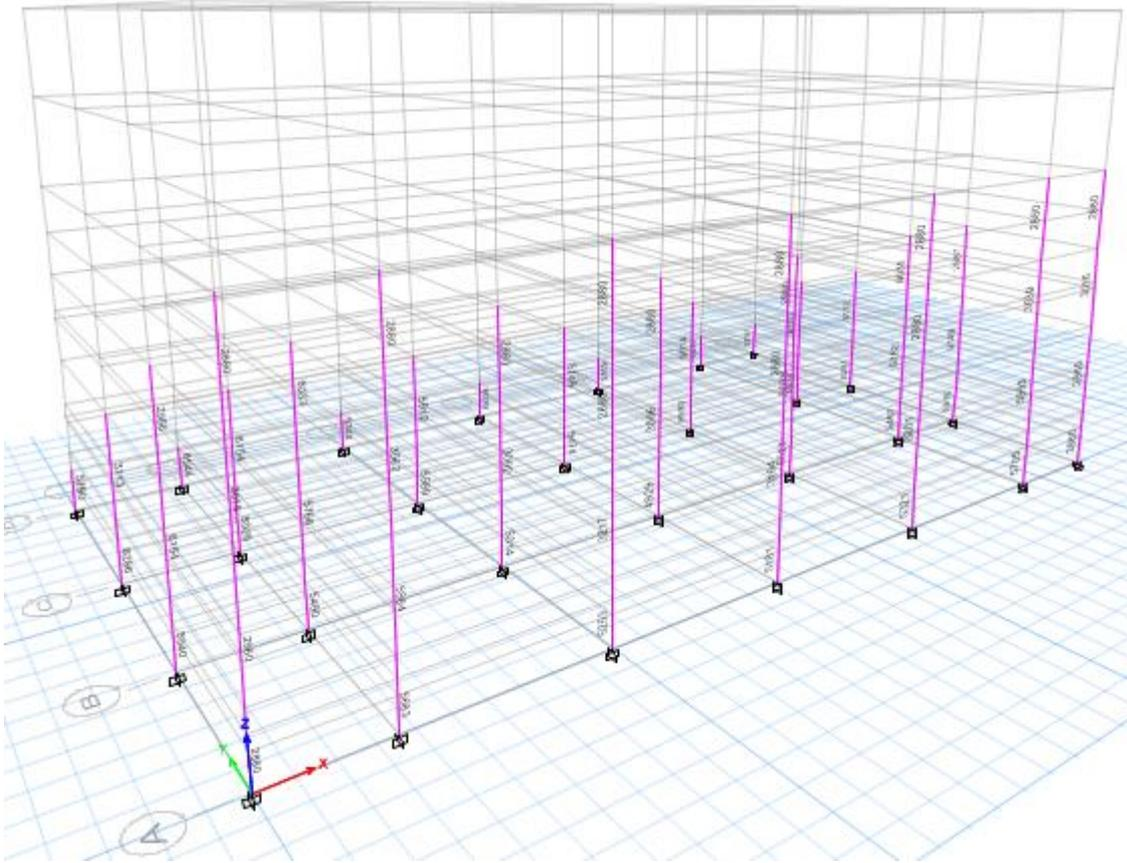
Figure 43: Column Reinforcement in Block B 1 & 3 (Columns only shown for clarity)
