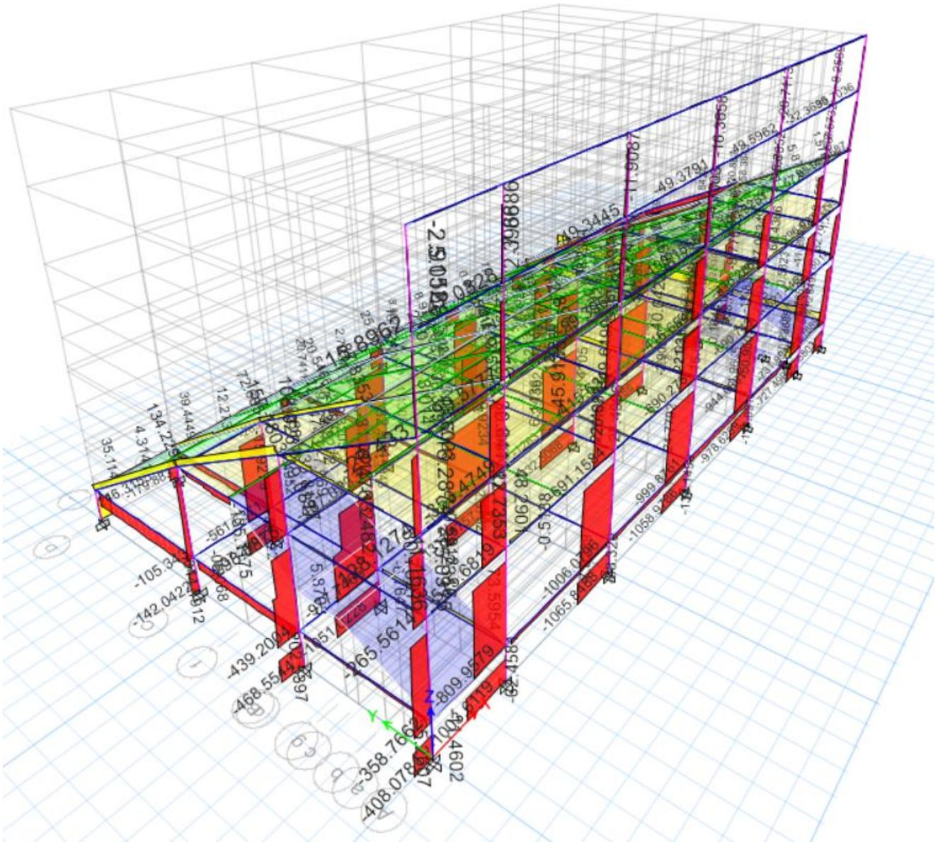
Figure 20: Axial force in Block B 1 & 3
