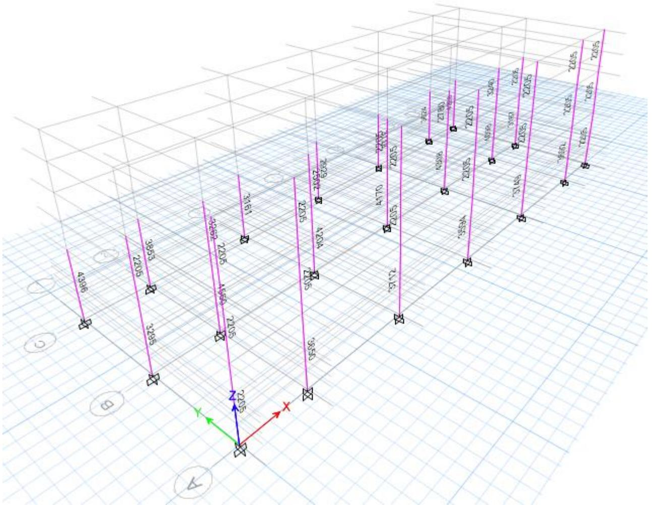
Figure 40: Column Reinforcement in Block A 1 & 3 (Columns only shown for clarity)
