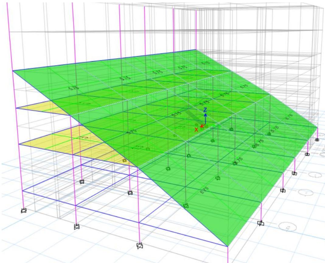
Figure 9: Floor Finish load (Block B 2)
