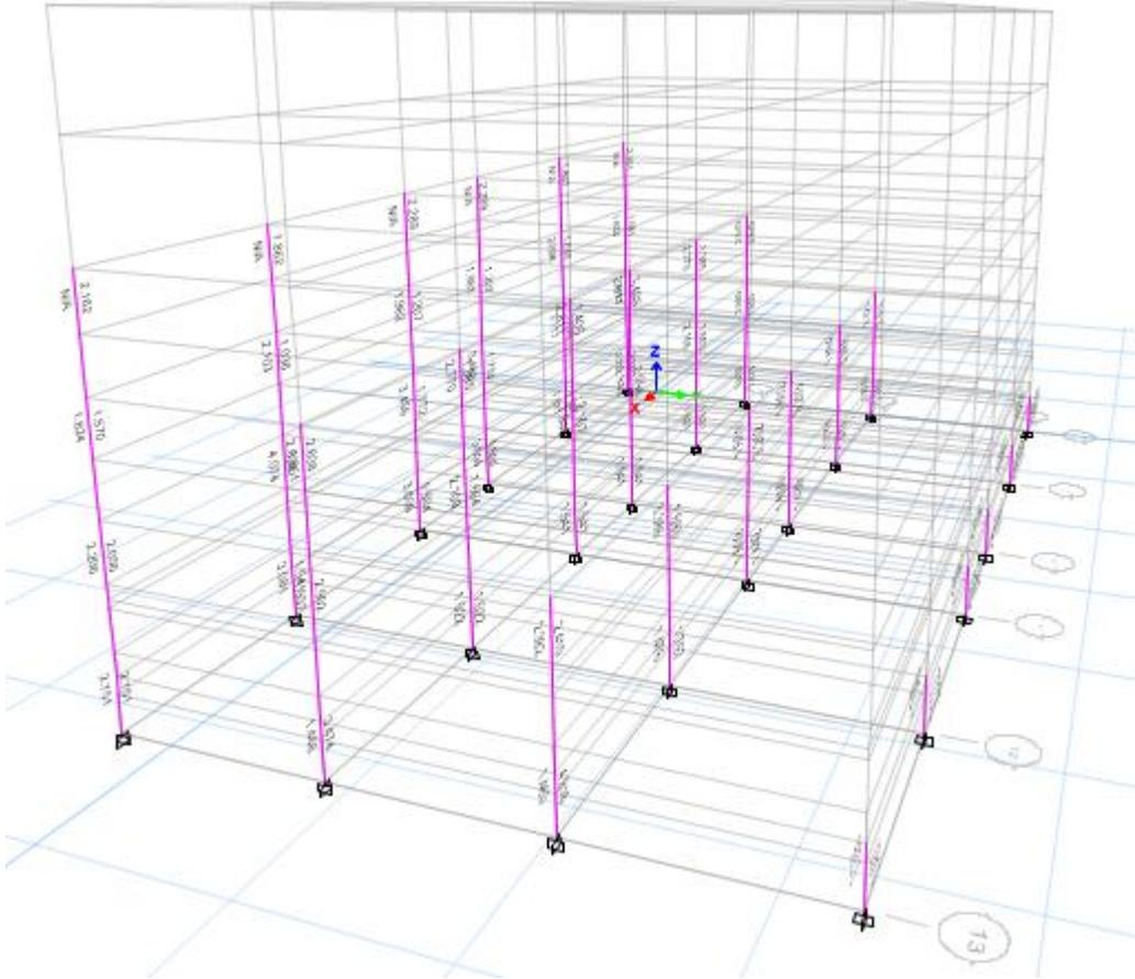
Figure 45: Column/ Beam Capacity Ratio in Block B 2(Columns only shown for clarity)
