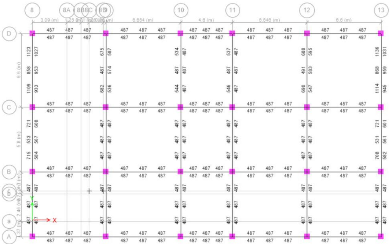
Figure 36: Sample Reinforcement at First floor beam (Block B 2)
