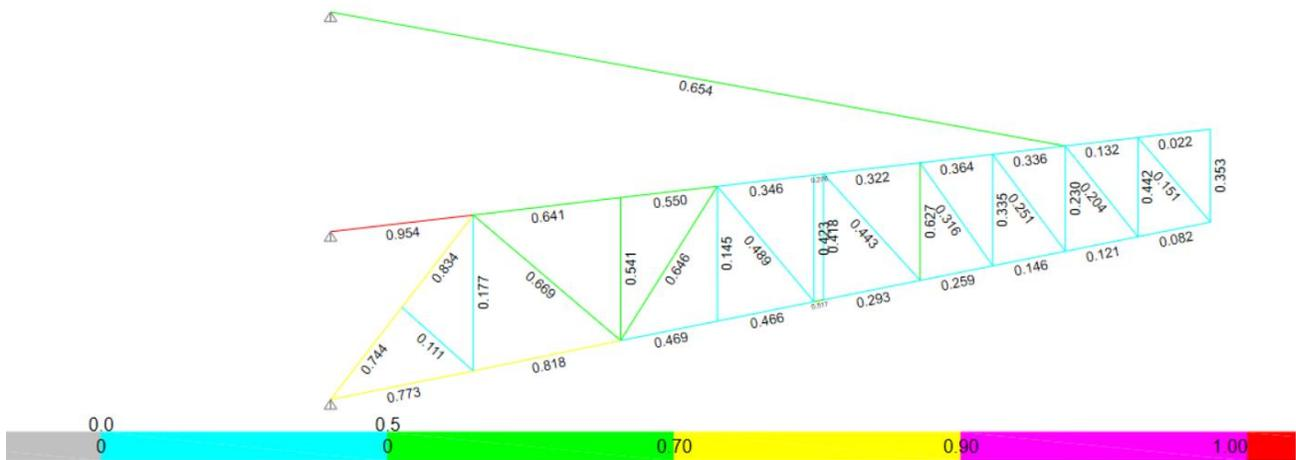
**Figure 7- 3: Design utilization ratio in truss**
