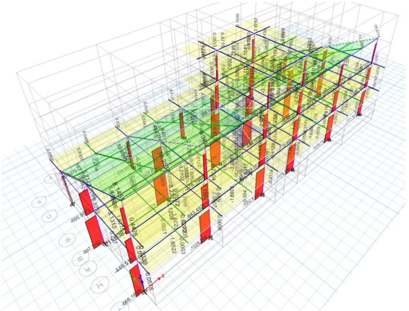
Figure 19: Axial force in Block A 2
