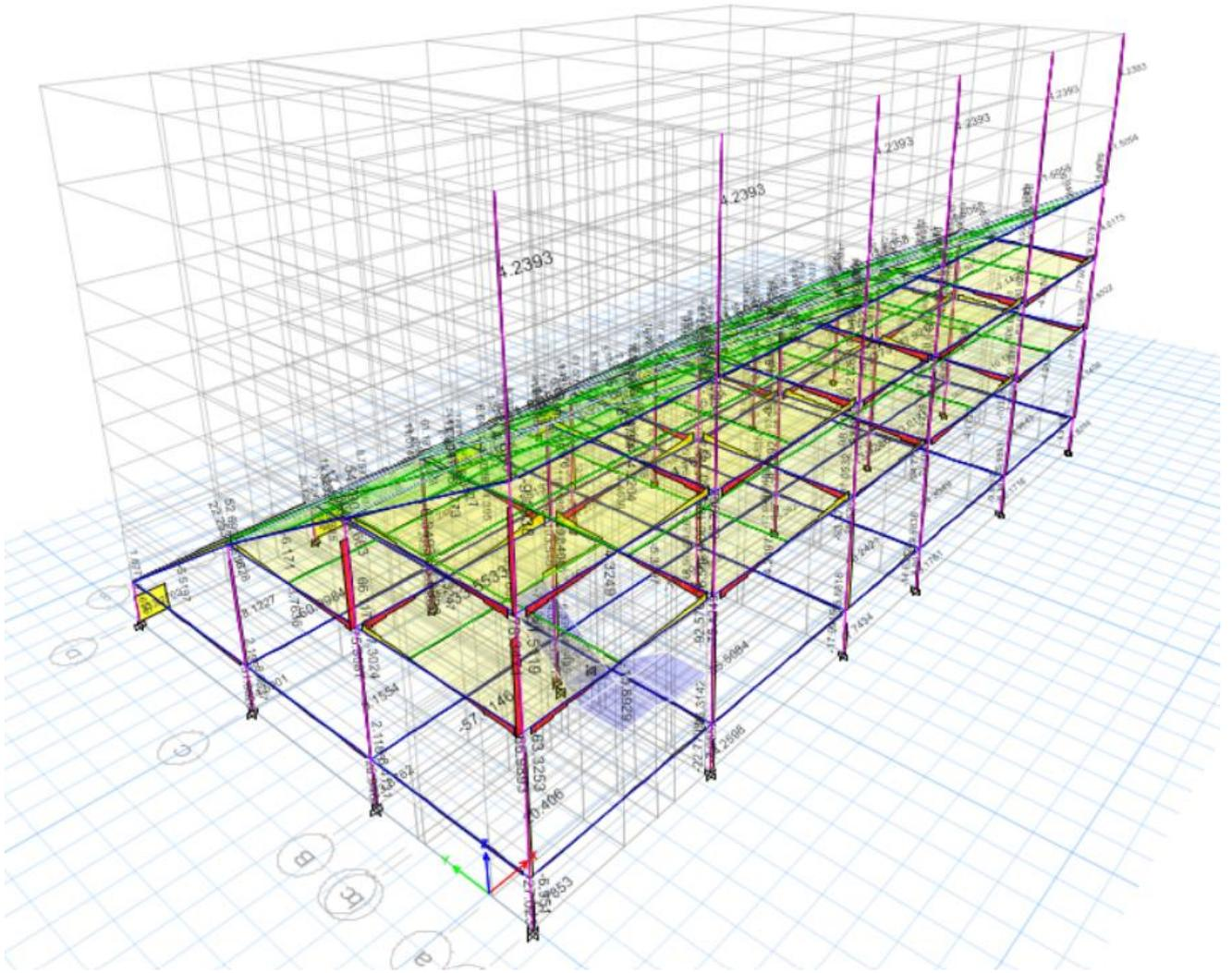
Figure 29: Shear Force Diagram in Block B 2
