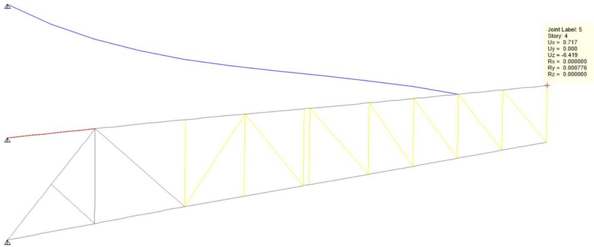
**Figure 6- 1: Deformed shape of the truss (DL+LL)**
