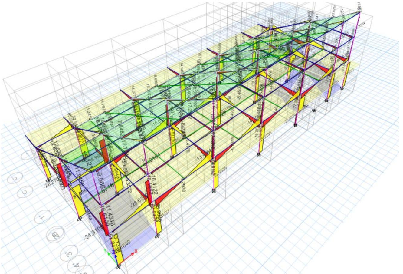
Figure 26: Shear Force Diagram in Block A 1 & 3
