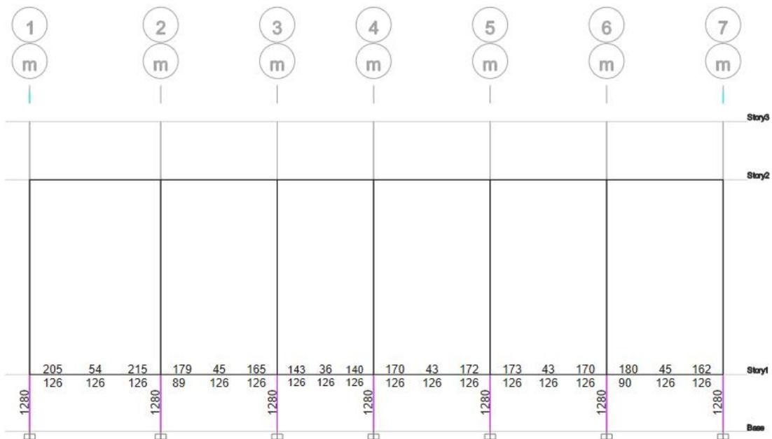
Fig: Reinforcement details along Grid M-M
