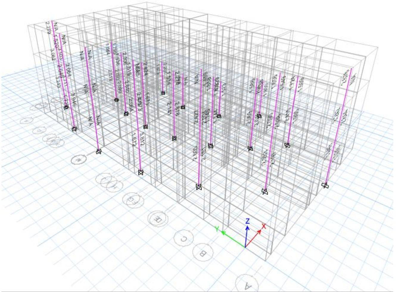
Figure 45: Column/ Beam Capacity Ratio in Block C(Columns only shown for clarity)
