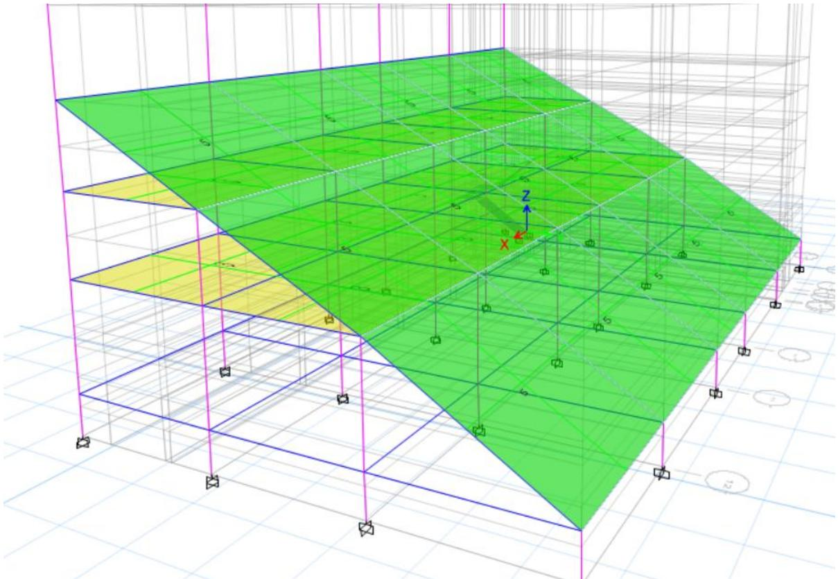
Figure 13: Sample Live Load < 3 KN/m<sup>2</sup> (Block B 2)
