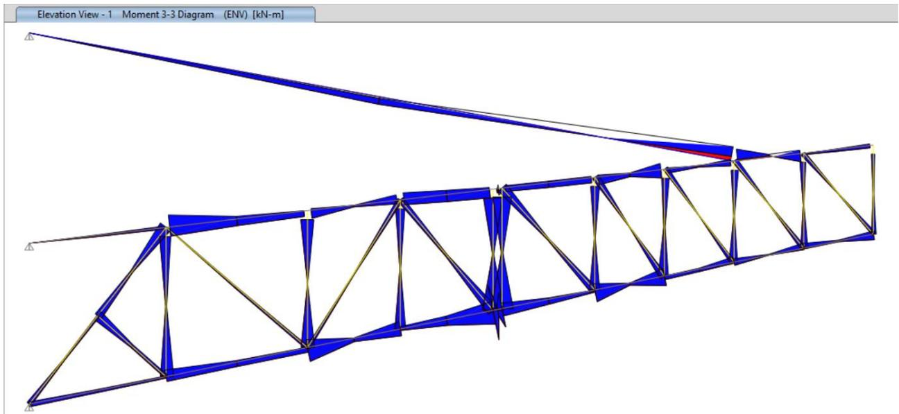
**Figure 6- 3: Envelope of M3-3 diagram**
