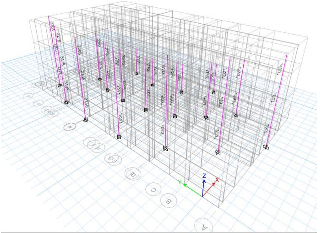
Figure 44: Column Reinforcement in Block C (Columns only shown for clarity)
