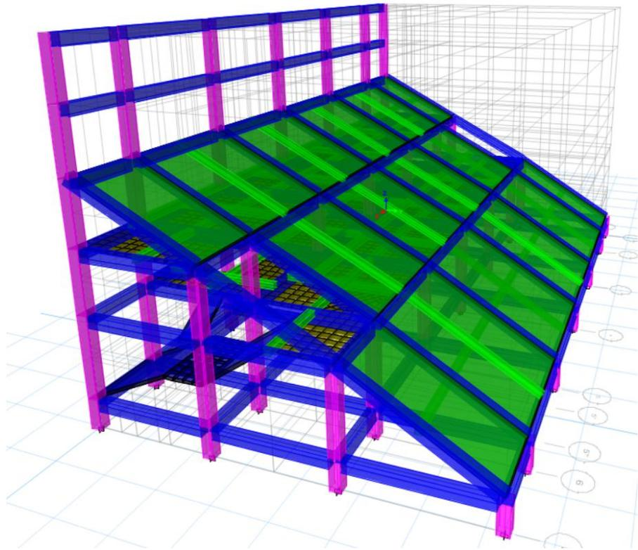
Figure 4: Finite Elemental Modeling in ETABS V19 (Block B 1 & 3)
