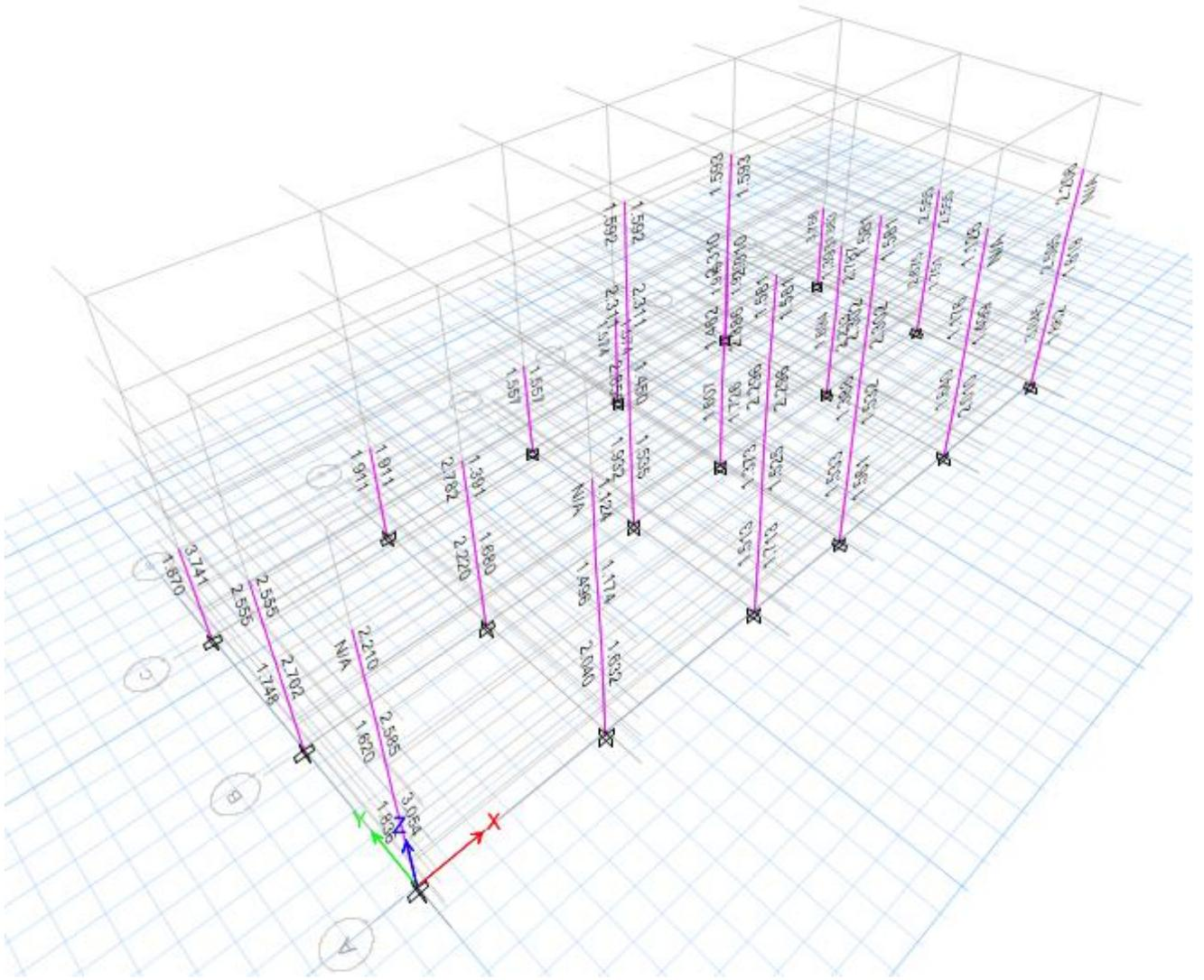
Figure 39: Column/ Beam Capacity Ratio in Block A2 (Columns only shown for clarity)
