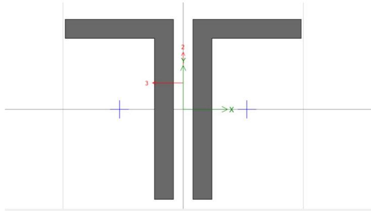
**Figure 7- 2: Double angle section ISA 100x65x8**
