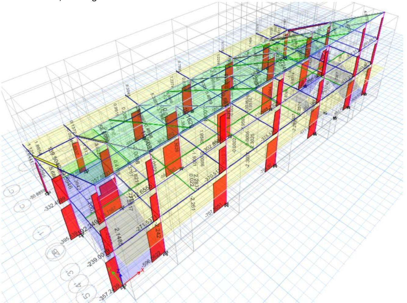
Figure 18: Axial force in Block A 1 & 3
