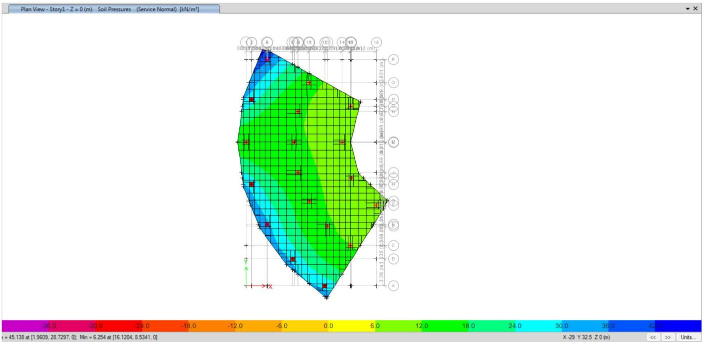
**Block C Soil Pressure < 80KN/m<sup>3</sup>**
