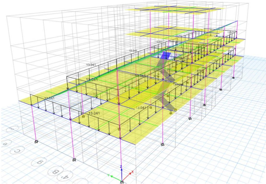
Figure 15: Sample Wall Load (Block A 2)
