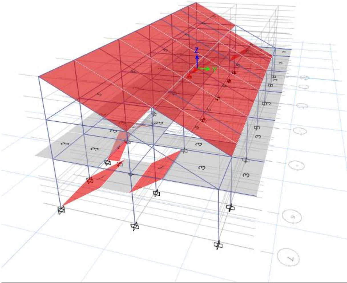
Figure 10: Sample Live Load  $< 3 \text{ KN/m}^2$  (Block A 1 & 3)
