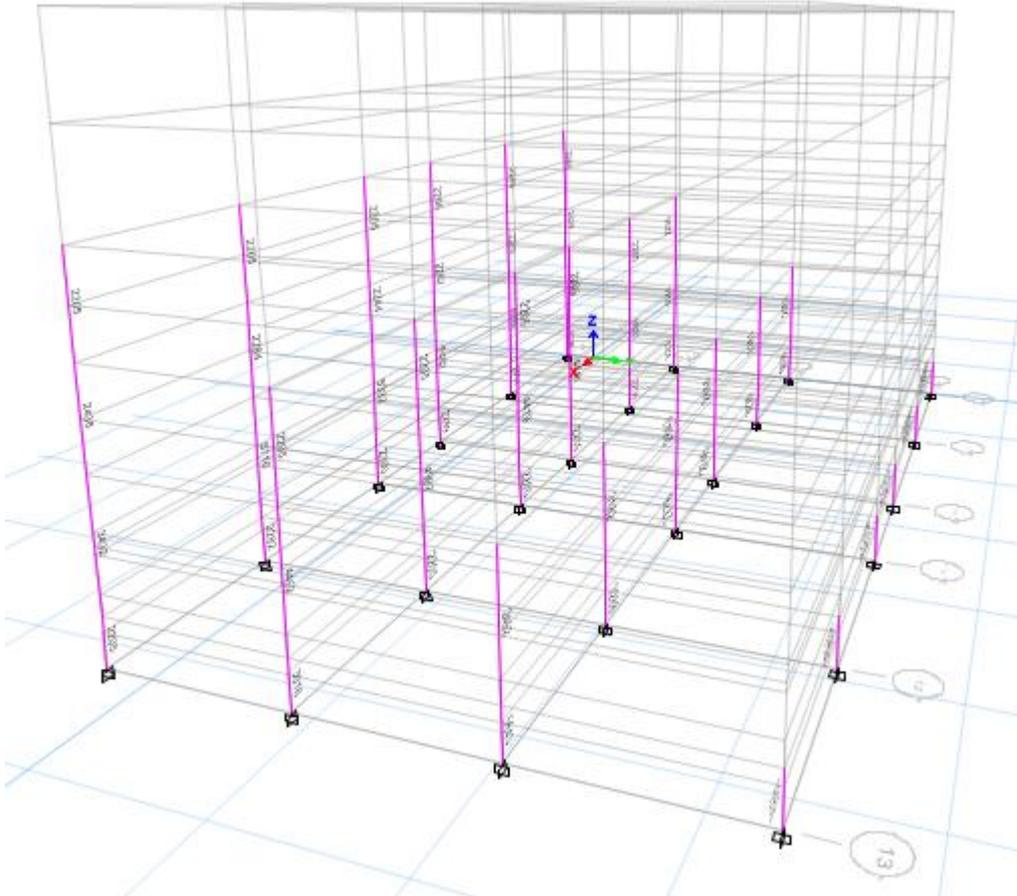
Figure 44: Column Reinforcement in Block B 2 (Columns only shown for clarity)
