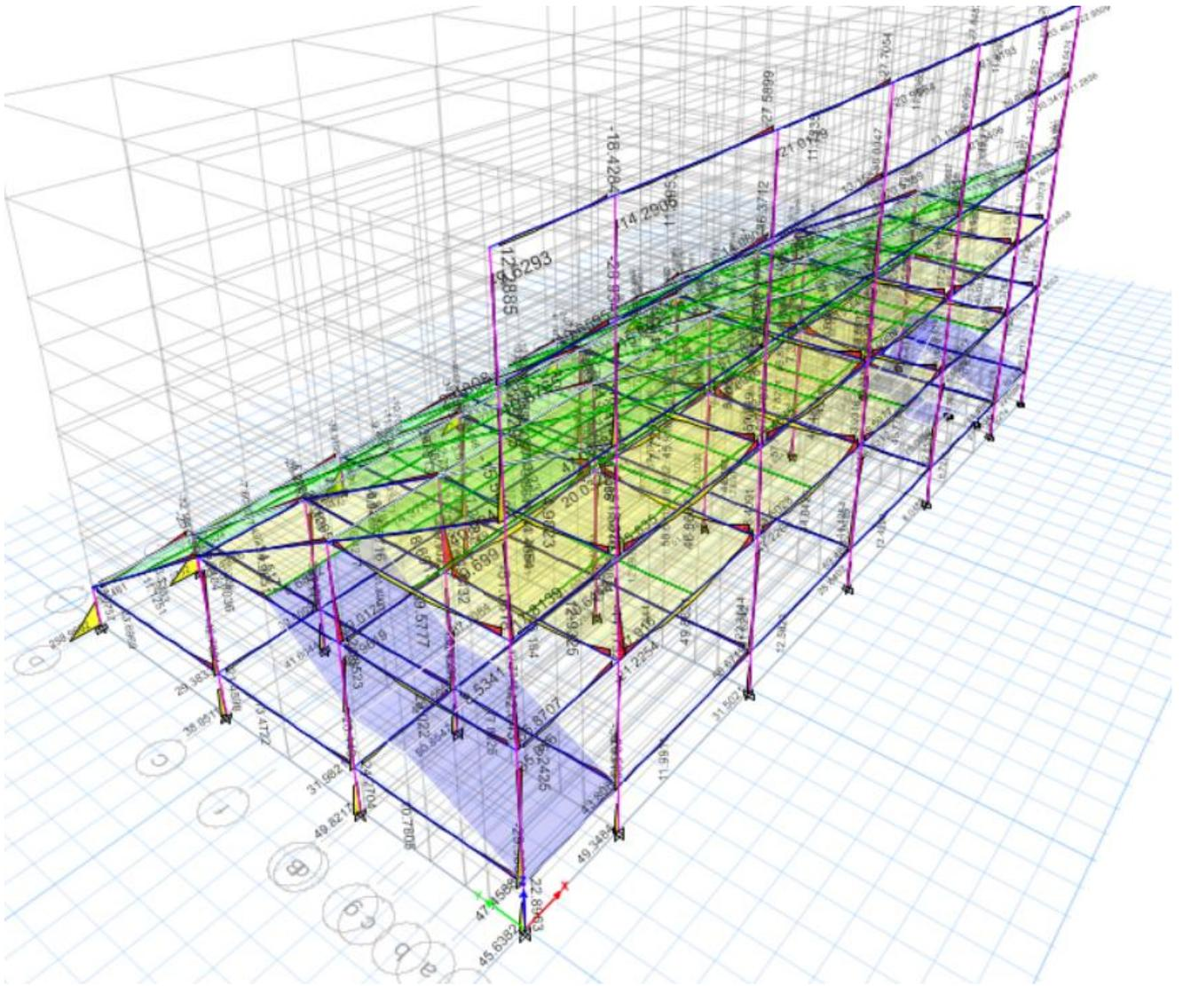
Figure 24: Bending Moment Diagram in Block B 1 & 3
