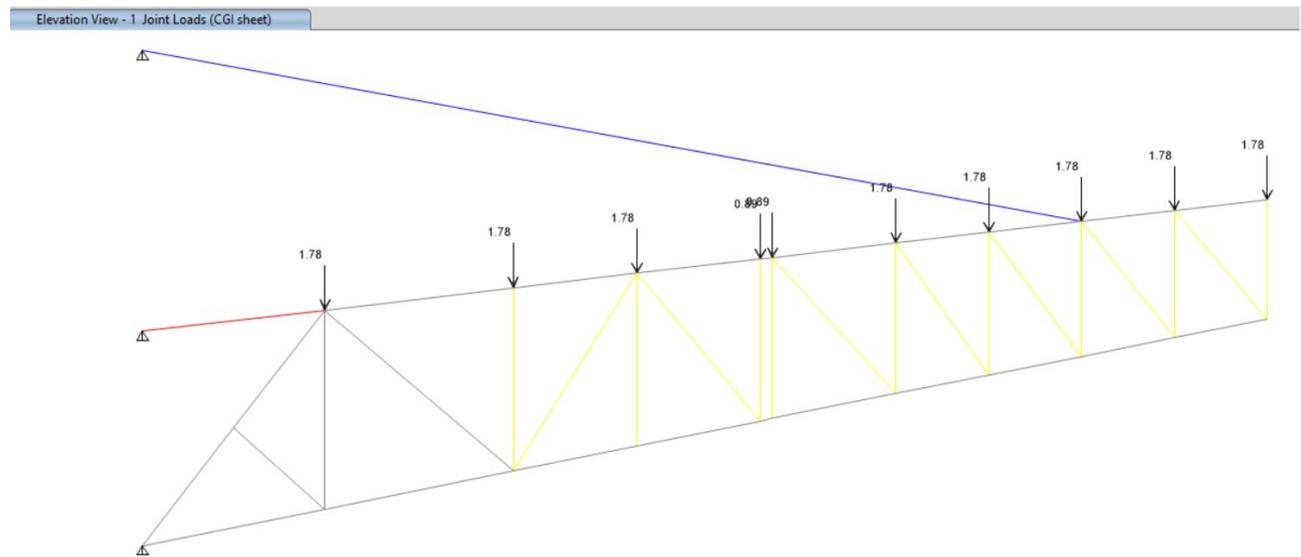
**Figure 4- 1: Application of joint load at each joint**
