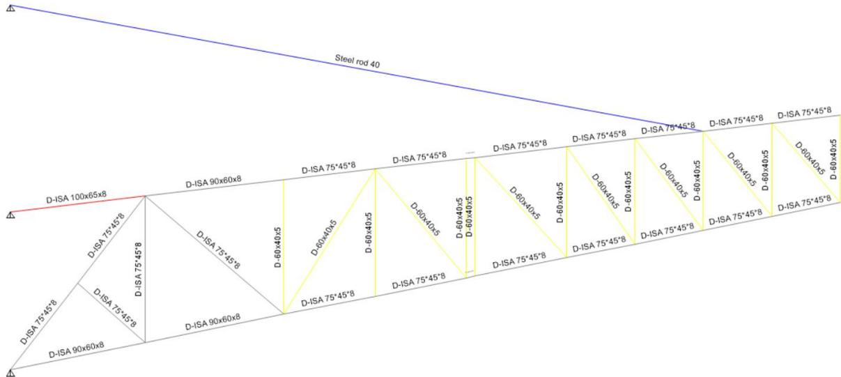
Figure 7- 1: Member details of roof truss
