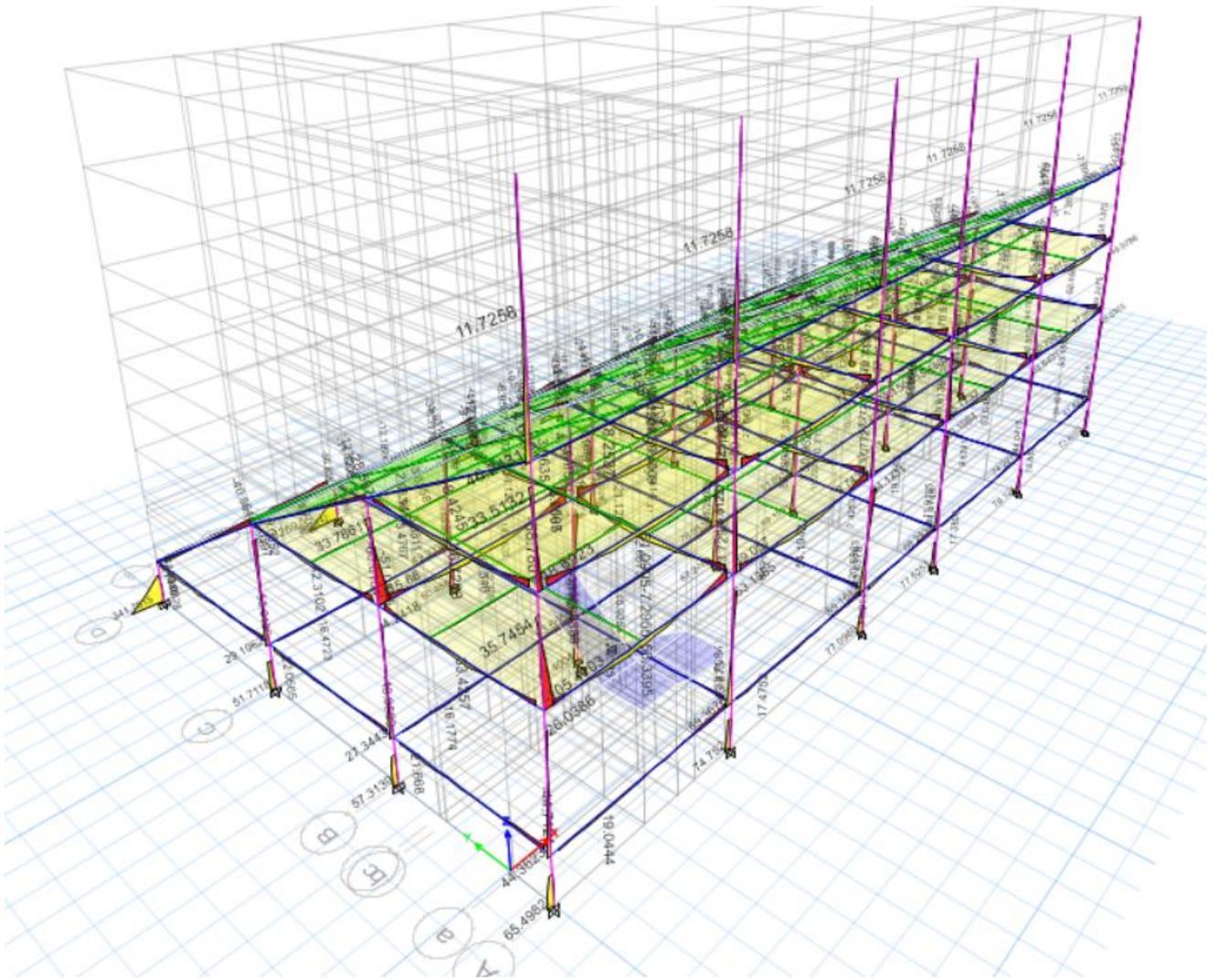
Figure 25: Bending Moment Diagram in Block B 2
