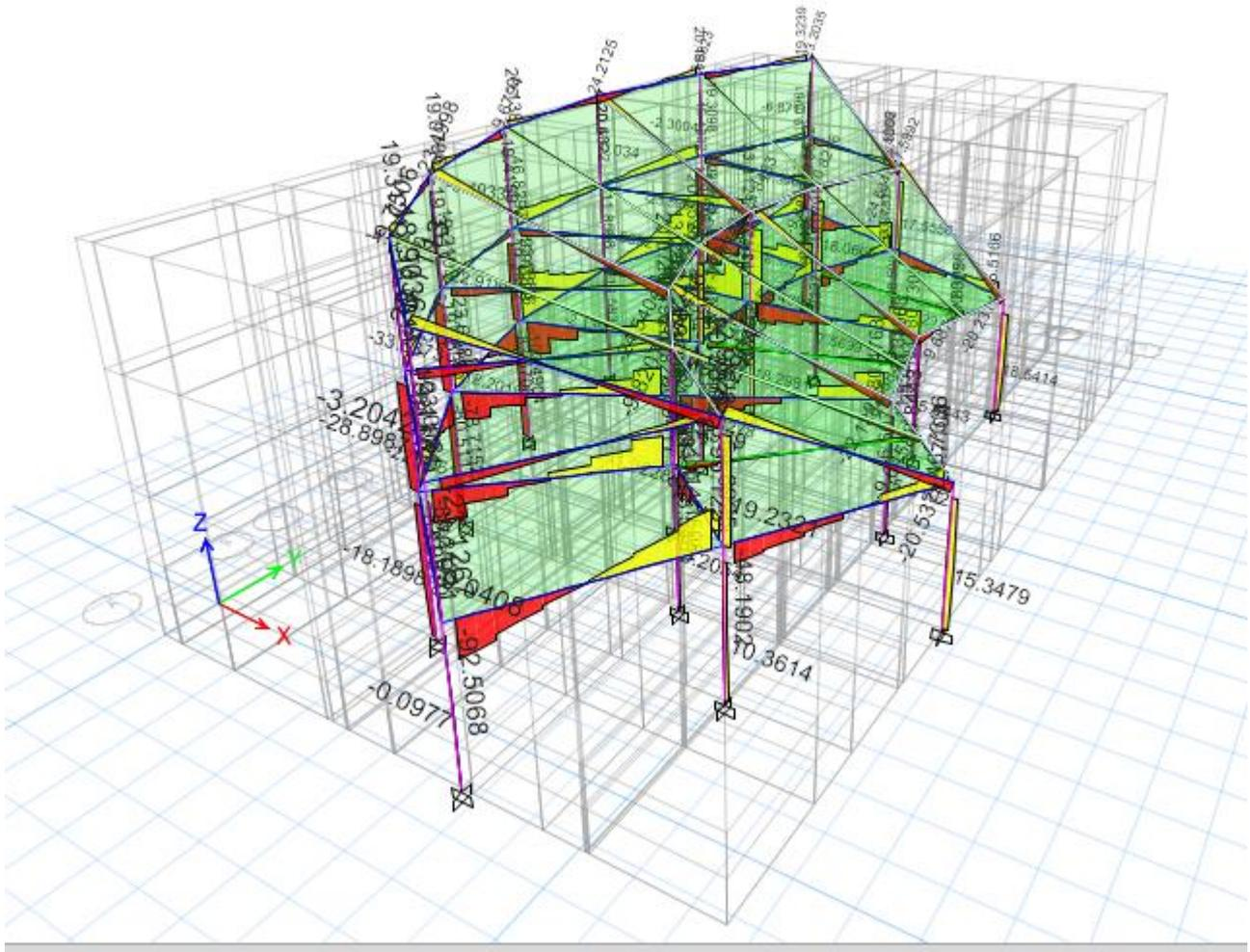
Figure 29: Shear Force Diagram in Block C
