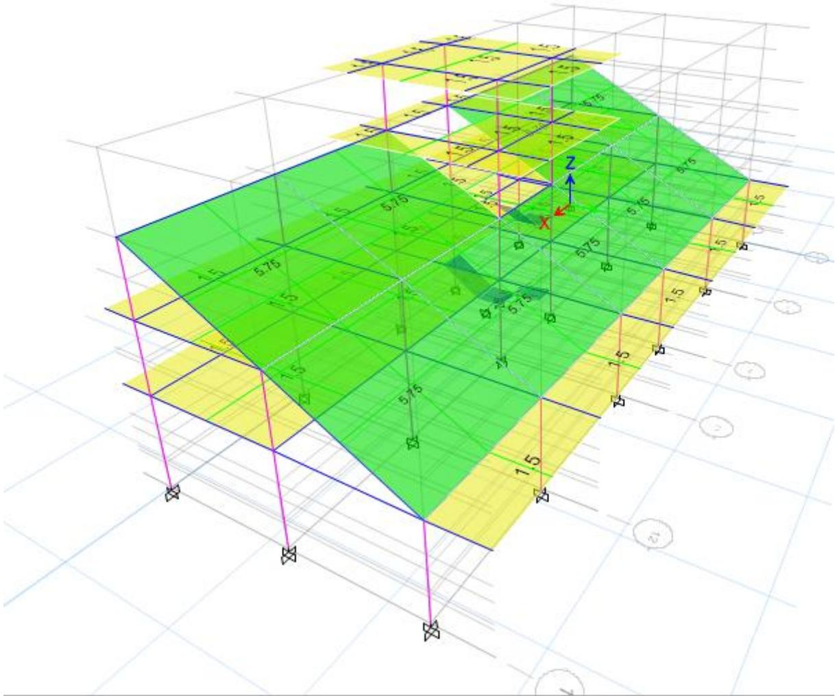
Figure 7: Floor Finish load (Block A 2)
