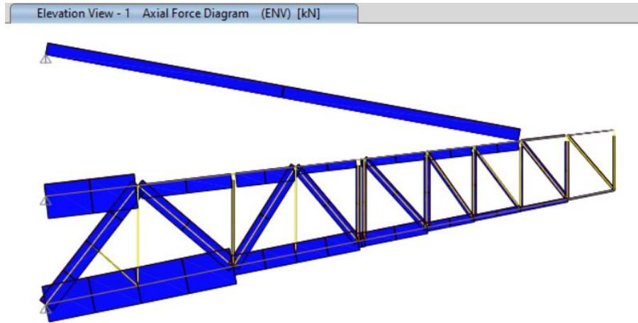
**Figure 6- 2: Envelope of axial force diagram**
