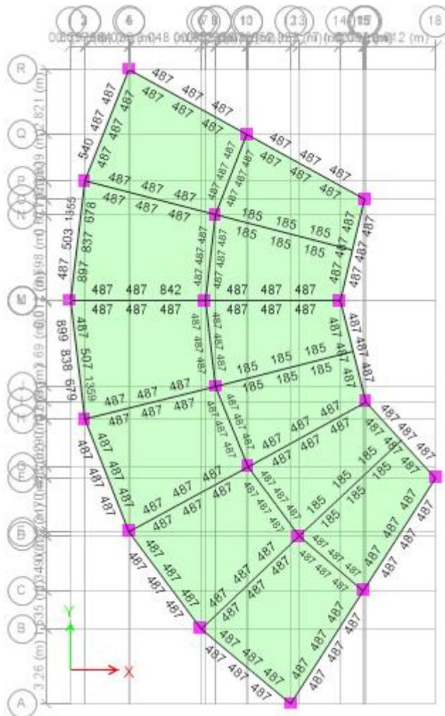
Figure 37: Sample Reinforcement at First floor beam (Block C)
