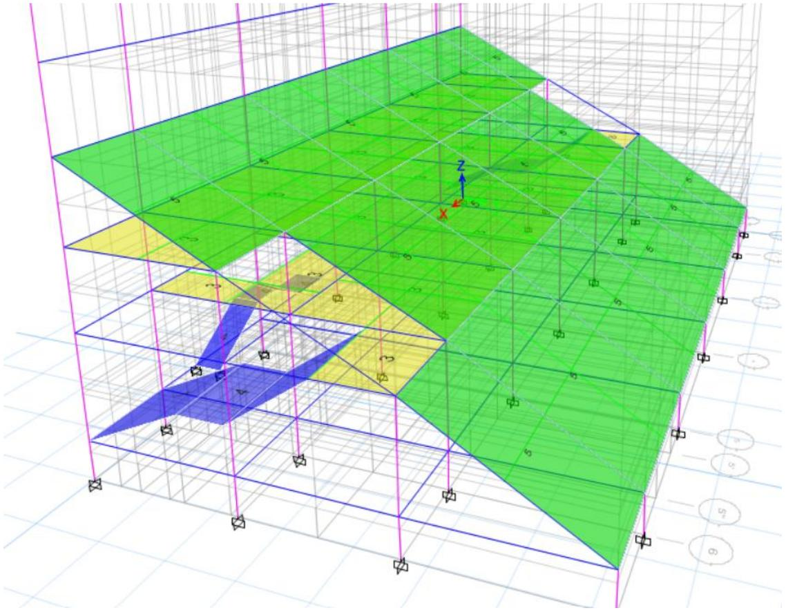
Figure 12: Sample Live Load < 3 KN/m<sup>2</sup> (Block B 1 & 3)
