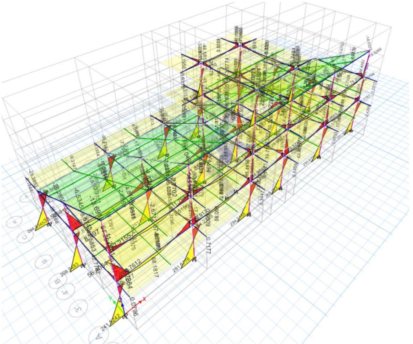
Figure 23: Bending Moment Diagram in Block A 2
