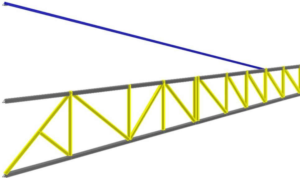
Figure 5- 1:3D view of FEM Model OF ROOF TRUSS
