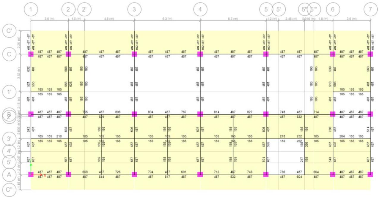
Figure 35: Sample Reinforcement at First floor beam (Block A 1 & 3)
