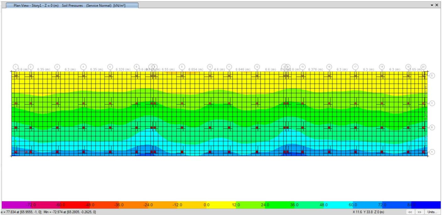
**Block B Soil Pressure < 80KN/m<sup>3</sup>**
