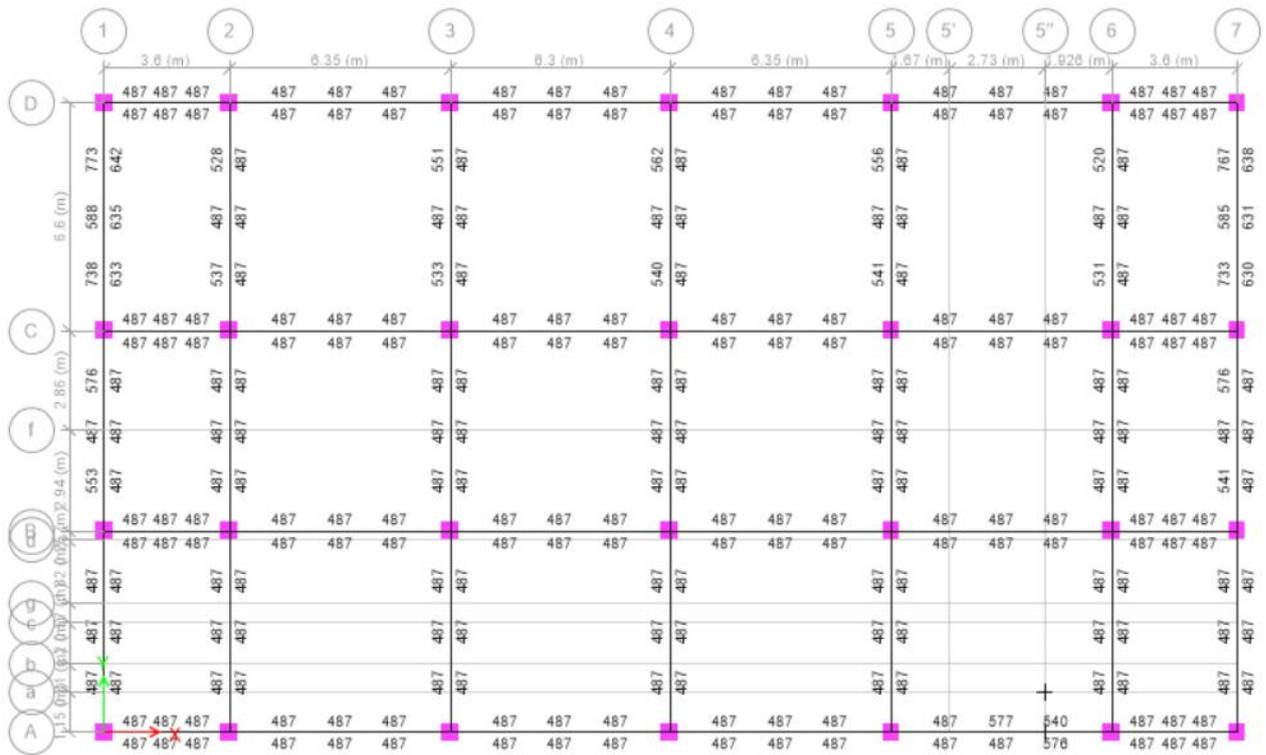
Figure 37: Sample Reinforcement at First floor beam (Block B 1 & 3)
