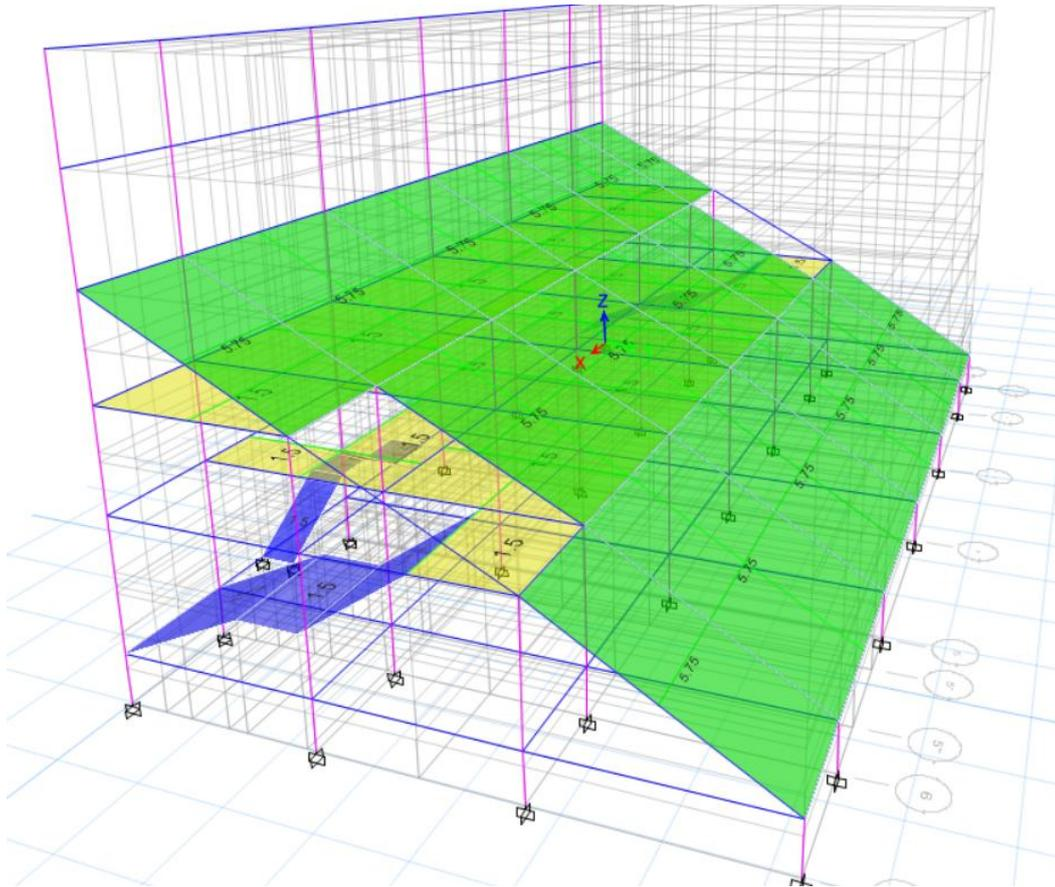
Figure 8: Floor Finish load (Block B 1 & 3)
