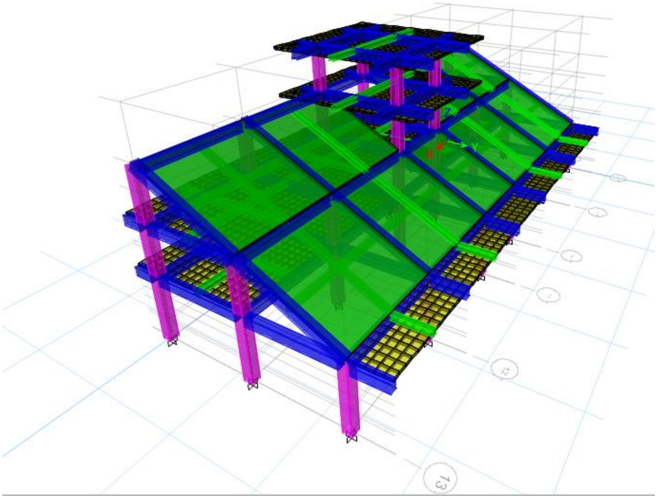
Figure 3: Finite Elemental Modeling in ETABS V19 (Block A 2)
