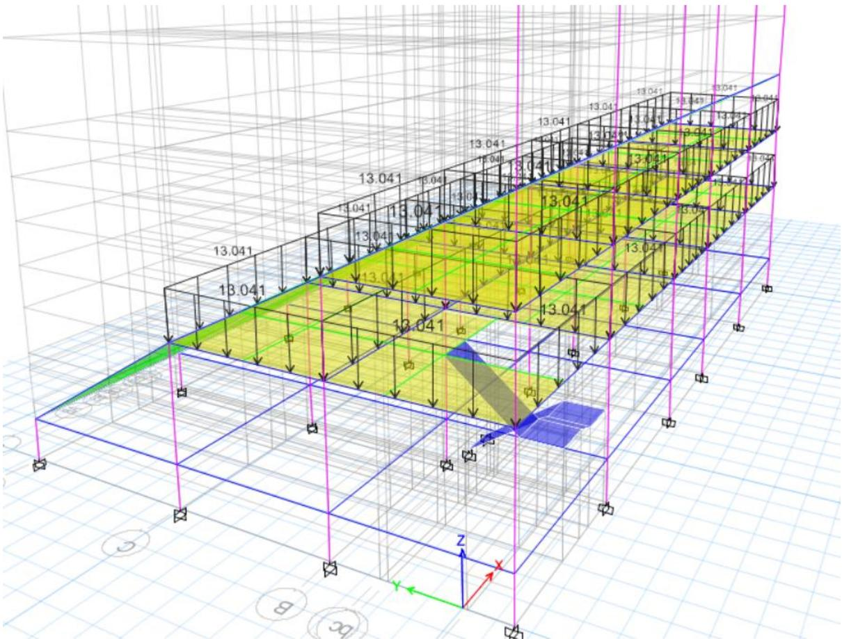
Figure 17: Sample Wall Load (Block B 2)
