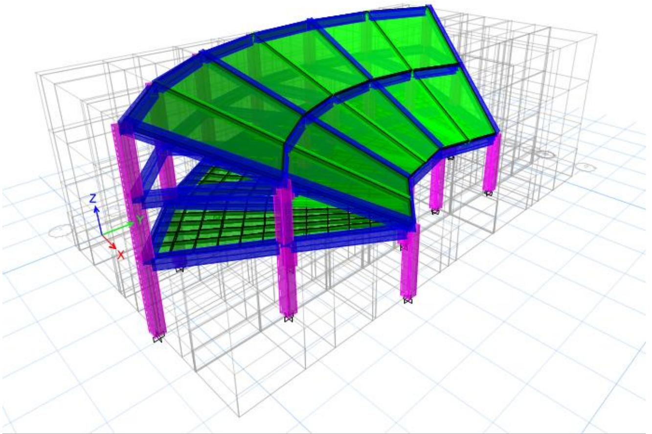
*Figure 5: Finite Elemental Modeling in ETABS V19 (Block C)*
